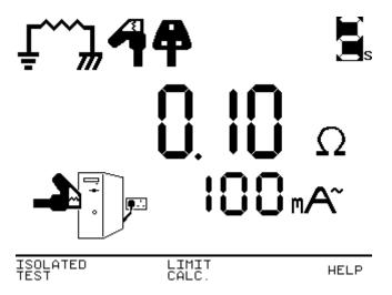
5. Disconnect the earth bond probe from the previous point and connect it to a conductive part of the EUT enclosure.
