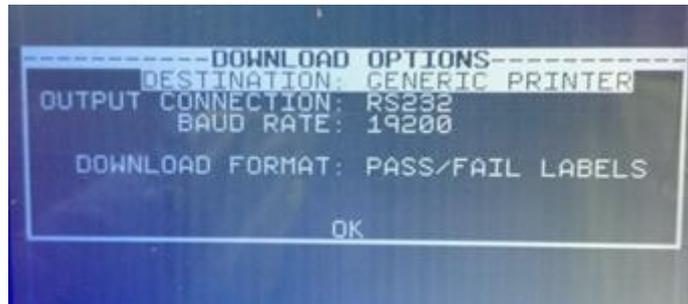
22. Connect the printer to the scanner using the serial cable provided with the printer ensuring to connect the side that says 'PRINTER END' to the printer.
