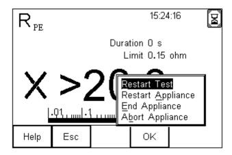
By selecting Restart Test the user can now go back to the beginning of the Earth Bond Test, however this time they will notice that the F3 key on the tester now has an active function calc.
