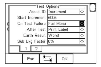
When performing a test where the nominal resistance is greater than the pre-defined pass limit the tester will fail the equipment, however the following menu will appear.
