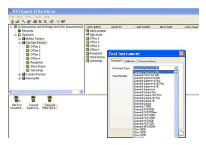
6) PATGuard is now ready to send data to the Seaward test instrument. Do not press OK until the PrimeTest 350 has been set to receive the upload.
