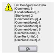
10. Press "OK" to accept the upload. This uploaded data can then be used from the dropdown selections when setting up / using your Apollo 600+
