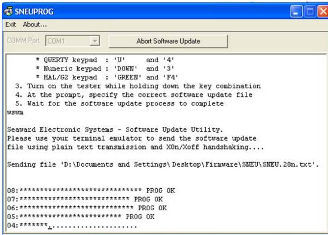
Do NOT interrupt the data transfer to the tester. If this transfer is aborted, the tester operating program will not be fully updated, resulting in probable failure of the tester, even though this may not be obvious on a short test. If the data transfer is aborted a successful code loading MUST take place before the tester is used again.
