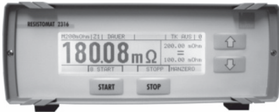
Front Panel with backlit LCD display and integral membrane keypad with tactile feedback
