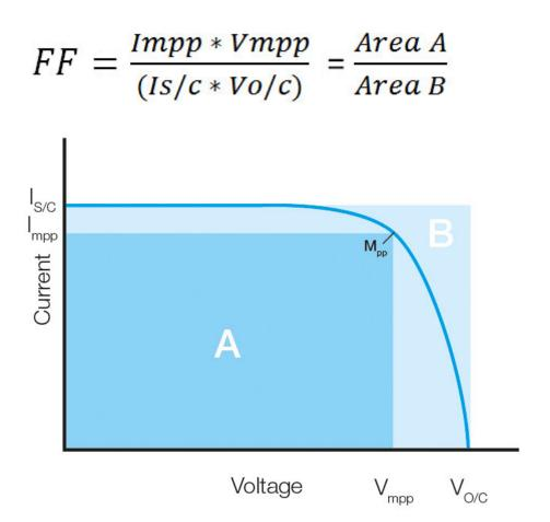
The Fill Factor is essentially a measure of the efficiency of a PV module, the theoretical maximum value depending on factors such as the type of silicon used to construct the module. However, deviation from the expected value or changes in Fill Factor can provide an indication that a fault is present.
