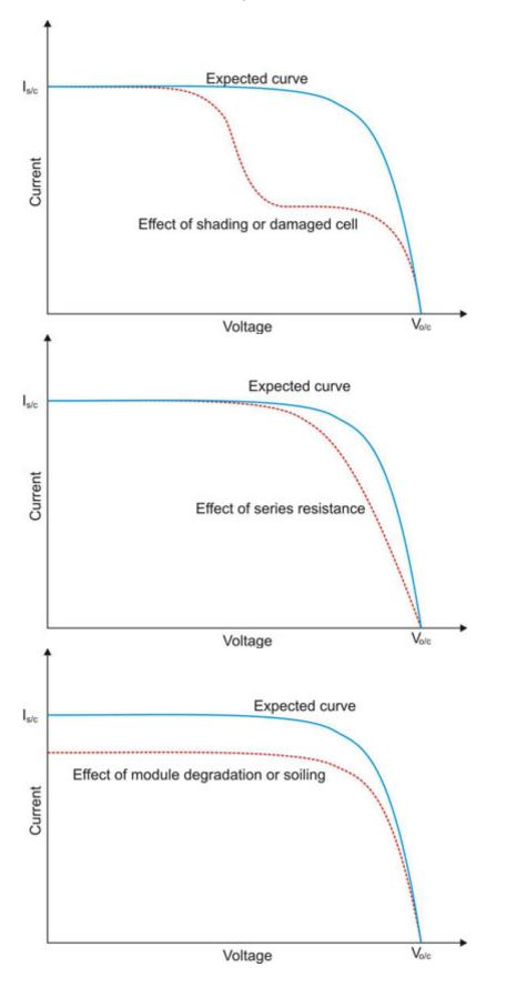
15-18 Bracken Hill, South West Industrial Estate, Peterlee, County Durham, SR8 2SW, United Kingdom t: +44 (0) 191 586 3511 | f: +44 (0) 191 586 0227 | e: sales@seaward.com seaward.com The I-V curve tracer can be used to as a diagnostic tool to identify, locate and rectify any of these problems.
