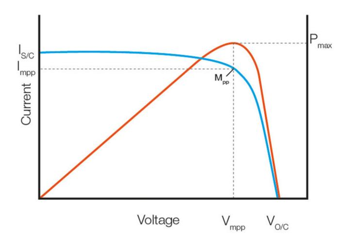
Power is the product of voltage and current and so the power vs voltage curve shown in figure 2 can be generated from the measured voltage and current data. The power vs voltage curve shows the point at which the power is a maximum (Pmax). The corresponding maximum power point Mpp is shown on the I-V curve. Loading the PV module such that the current is Impp and voltage is Vmpp will operate the PV module at the maximum power point (Mpp) and result in the maximum power generation.
