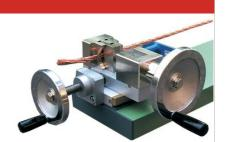
Measurement length: 1000mm. Clamping device: designed for cross sections of 1mm<sup>2</sup> to 1000mm<sup>2</sup>. Distance between voltage and current-clamp: 420mm. Dimensions (height x width x depth): 170mm x 2100mm x 250 mm. Weight: Approximately 25kg.
