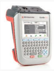
Note: The requirements of a formal visual inspection will vary according to the equipment being inspected and the environment in which it is used. The 'prompts' built into Seaward Portable Appliance Testers (Apollo 600, Supernova Elite, Europa Plus and PrimeTest range) are intended to provide guidance and should not be taken as a comprehensive list of items to be checked during a formal visual inspection.
