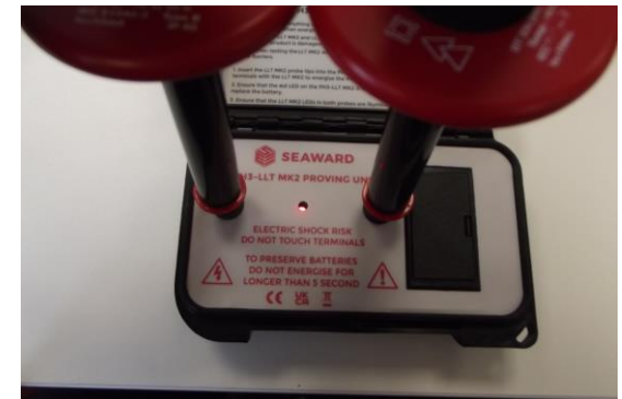
Image above shows PH3-LLT MK2 switched on when the right terminal is pushed down.
