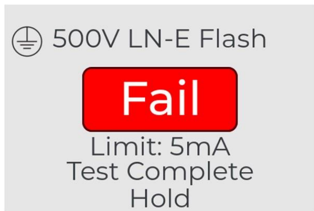
Figure 7: 500V LN-E Flash Fail
