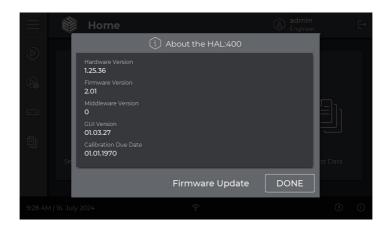
The resulting screen, above displays useful information about your HAL:400 including the hardware version, firmware versions. In addition a reminder function for the calibration due date will also be displayed.
