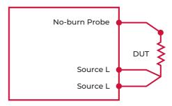
The No-Burn probe maintains the four wire measurement principle. It has a unique press and hold facility to ensure no marking on the product surface due to poor contact resulting in sparking. The probe also serves to provide the operator information via the inbuilt LED during the Earth Bond Test, with the following conditions:
