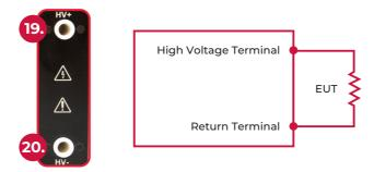
Connect the (Red) High Voltage test lead to the High Voltage Terminal (19) and ensure the plug is firmly connected into the socket.
