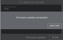
After completing the download, the HAL:400 will load the new firmware automatically. Upon completion the HAL:400 will require a restart in order to apply the updates.
