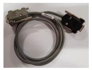
Connect the printer to the test equipment into the Serial port of the tester, ensuring the Grey end is connected to the printer (labelled as Printer End). For HAL series test equipment, ensure the cable is connected to the Printer port, identified with a printer icon.
