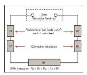
When measuring larger resistance values this additional lead resistance error can be ignored, but as you can see from the chart below, the error becomes significantly higher as the measured value decreases, and totally inappropriate below 100
