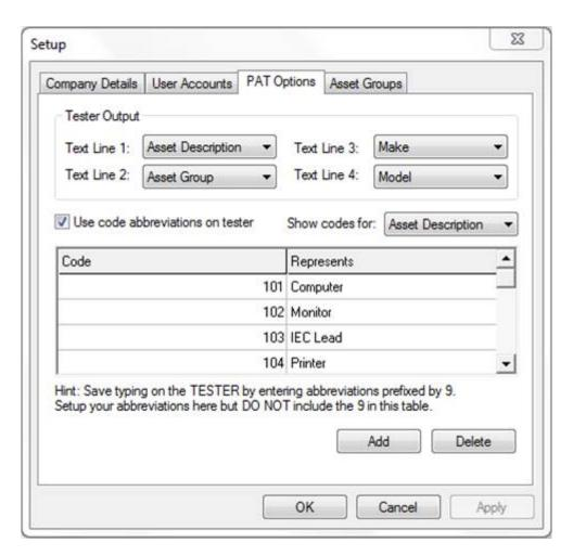
Note: When entering codes at the instrument, the 3 digit short code MUST be prefixed by a number 9. This is so that PATGuard 3 will recognise the value as a Short Code.
