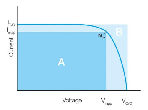
The Fill Factor is essentially a measure of the efficiency of a PV module, the theoretical maximum value depending on factors such as the type of silicon used to construct the module. However, deviation from the expected value or changes in Fill Factor can provide an indication that a fault is present.
