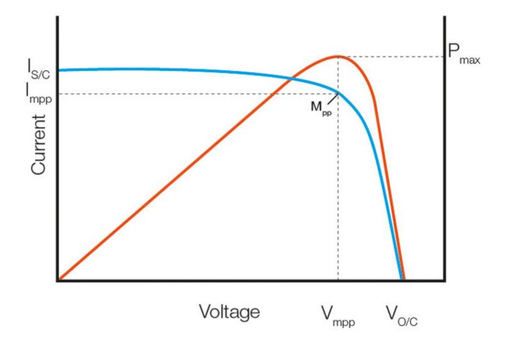
Power is the product of voltage and current and so the power vs voltage curve shown in figure 2 can be generated from the measured voltage and current data. The power vs voltage curve shows the point at which the power is a maximum (Pmax). The corresponding maximum power point Mpp is shown on the I-V curve. Loading the PV module such that the current is Impp and voltage is Vmpp will operate the PV module at the maximum power point (Mpp) and result in the maximum power generation.
