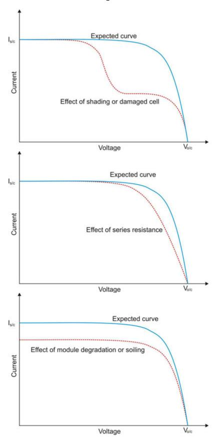
The I-V curve tracer can be used to as a diagnostic tool to identify, locate and rectify any of these problems.
